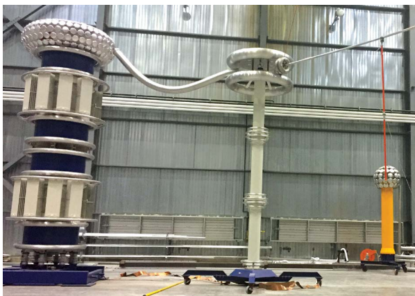
800 kV series resonant test system performing an AC withstand test on a live line working tool.
